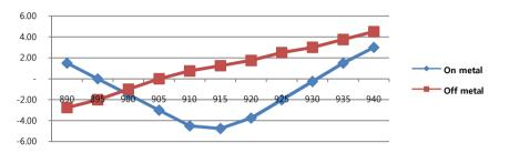
•BASIC L reads shorter by 50% or more off metal (or on non metal surface). It can be applied, therefore, only for metal application. For non metal application, please use PALLET.
