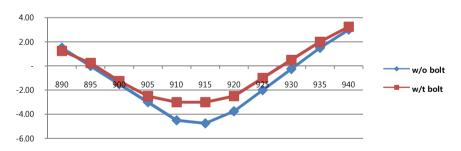
•BASIC I reads best without any metal bolt in two holes (located at center of both ends). With RF interference, metal bolts decreases read range by 15% or more. RFcamp recommends not using metal bolts, but 3M 300LSE adhesive or glue for maintaining optimum read performance. In case adhesive or glue can not be used, polycarbonate (or nylon) bolts is recommended.
